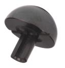
**MCPT FEATURES** 1144 STEEL, BLACK OXIDE FINISH - Heat-treated and hardened to R/C53 - 55(standard)
